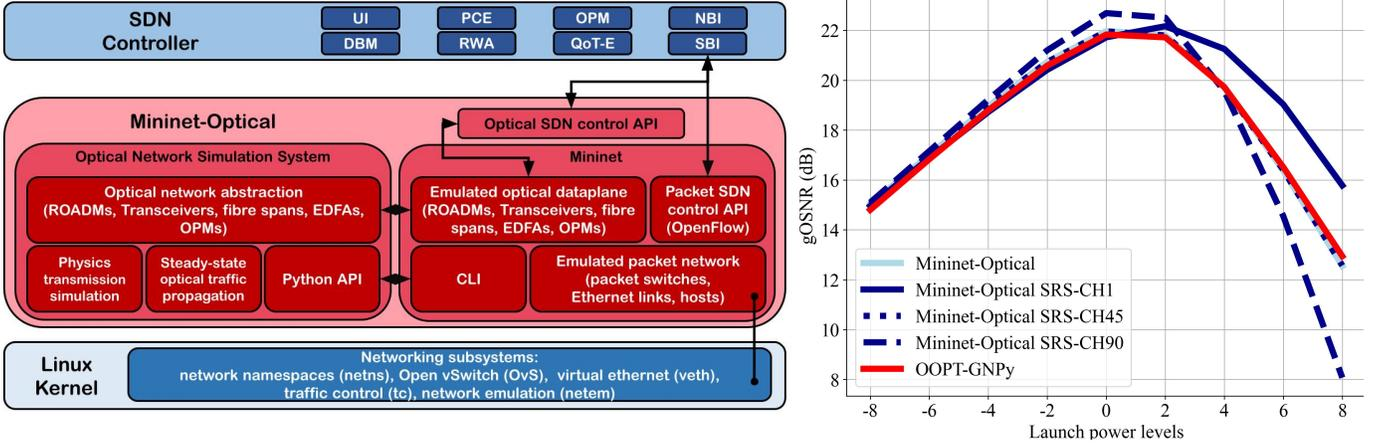
Fig. 1: (left) Mininet-Optical architecture diagram. (right) gOSNR performance comparison between the OOPT-GNPy Project [12] and Mininet-Optical (red and light blue curves, respectively) and Mininet-Optical with SRS modeling (dark blue curves) for the first, center, and last channels in a 90 C-band channel transmission.
