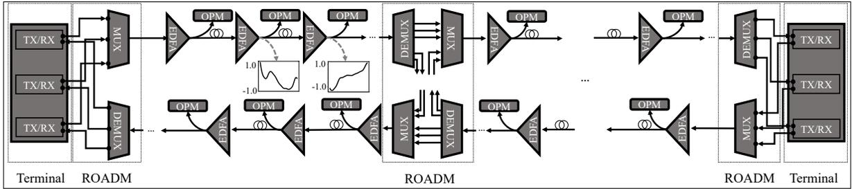
Fig. 2: Linear topology modeled with Mininet-Optical.
