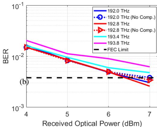
**Fig. 4:** Received power versus BER for skew (un)compensated 56 Gbd PAM-8 at various frequencies.
