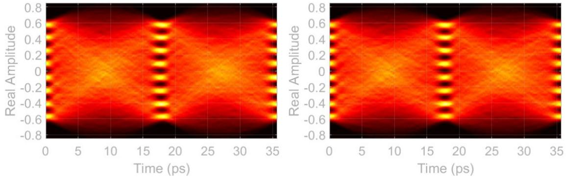
**Fig. 3:** 56Gbd PAM-8 eye diagrams exhibiting skew (a) and with receiver skew compensation (b).
