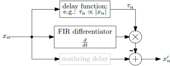
Fig. 2: Skew compensation structure.
