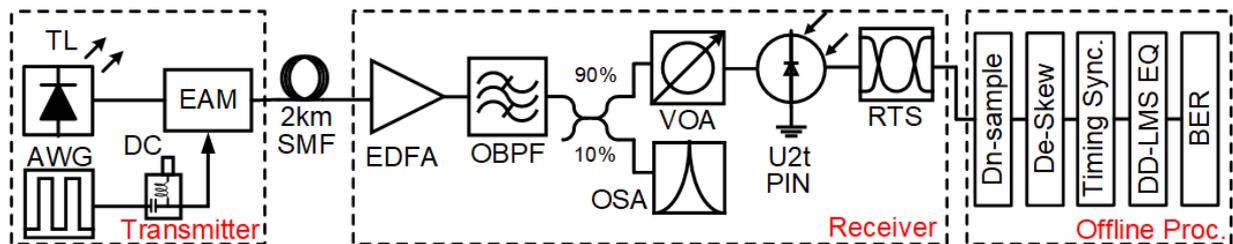
Fig. 2: 56Gbd PAM-8 transmission experimental test-bed.
