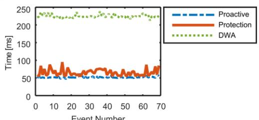
Fig. 5. Service restoration time for the protection mechanism and the DWA through the implemented SDN
