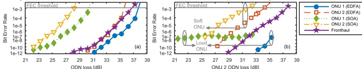
Fig. 3. BER of 10Gb/s PON downstream as a function of the ODN loss (a) and upstream as a function of ONU 2 ODN loss (b) for the two amplifier node designs and BER of the fronthaul channel as a function of the ODN loss.
