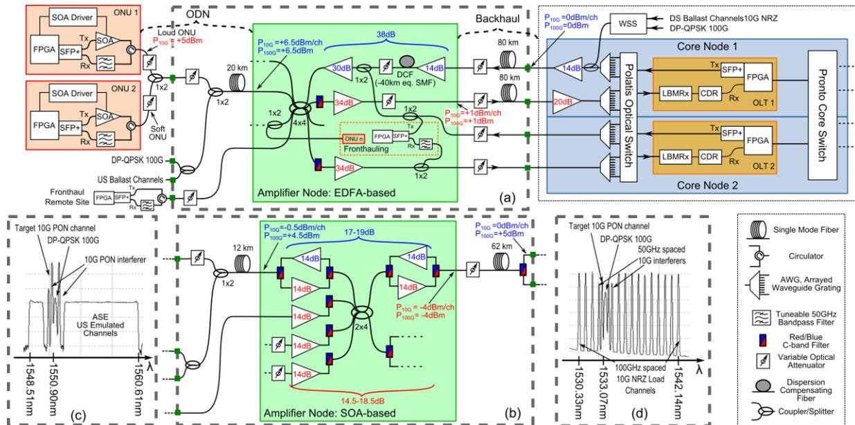
Fig. 2. Physical layer experimental setup with (a) EDFA-based and (b) SOA-based amplifier node
