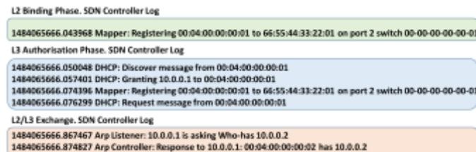
Fig. 4 SDN Controller log of Service Registration
